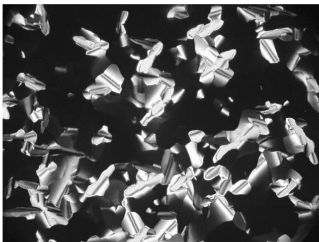
FIGURE 3 Microphotograph of the columnar mesophase of the melamine 1 in mixture with two equivalents of the benzoic acid 2 between crossed polarizers.
