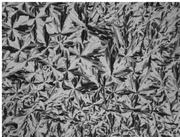
FIGURE 2 Optical texture of the induced mesophase of the equimolar composition 1/2 between crossed polarizers.
